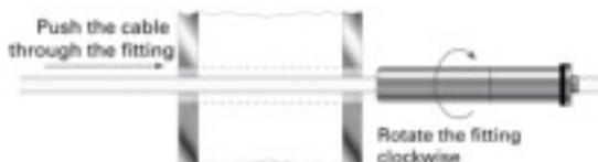
F. Push the pull-lock fitting along the cable and into the hole in your terminating post. While holding the pull-lock fitting against the end post, firmly pull the excess cable through the pull-lock to remove as much slack in the cable as possible. It is important to get the cables as tight as possible before using the threaded cable receiver to tension the cables. If needed use a pair of pliers.
